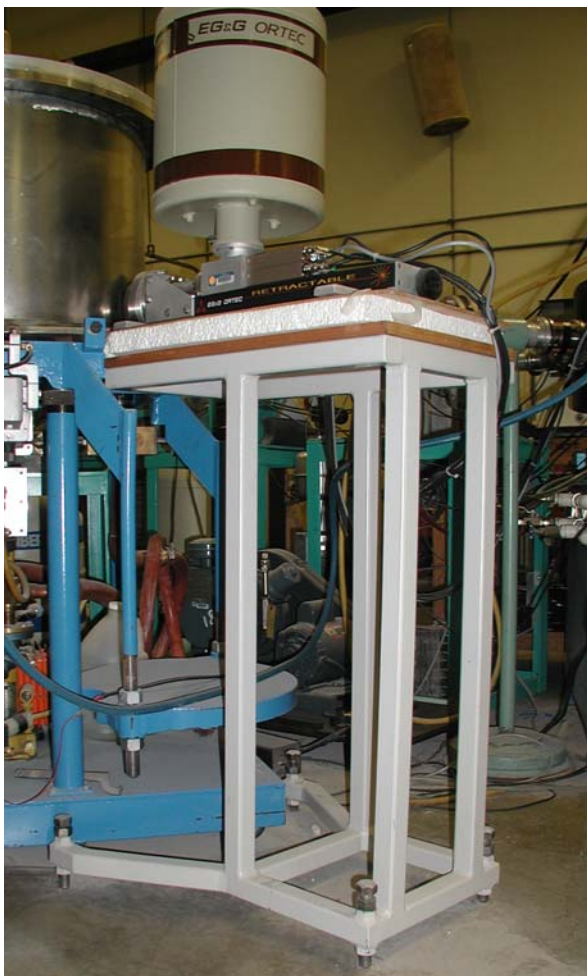
Figure 9: X-ray detector atop detector mounting table
