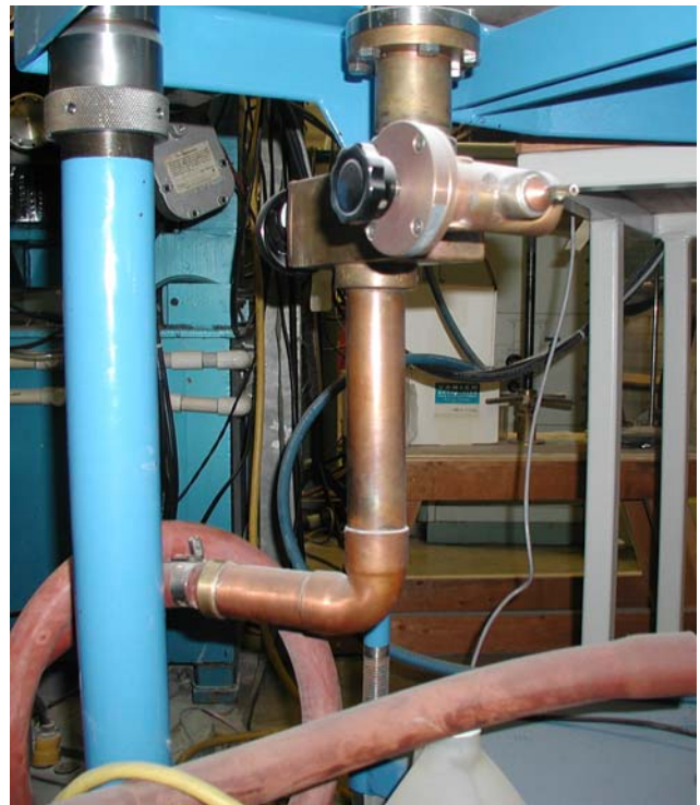
Figure 6: Photograph of copper pipe and helium intake spigot
